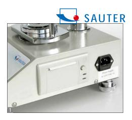
Manual test stand for tensile and compressive testing of springs, medium version from 50 N up to 500 N
